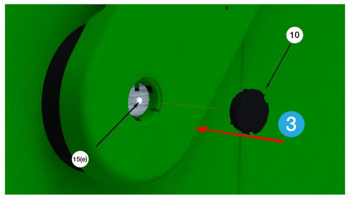
Step 3 – Put the cork on the hole of the lid (position .3).
